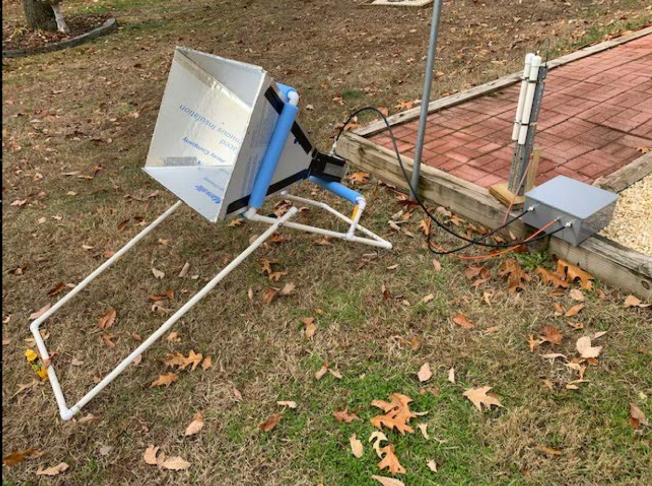
Continuum Observation - 1420.405 MHz - 1.6 MHz bandwidth - Horn antenna - 180az/70alt - Severn, MD All times local
